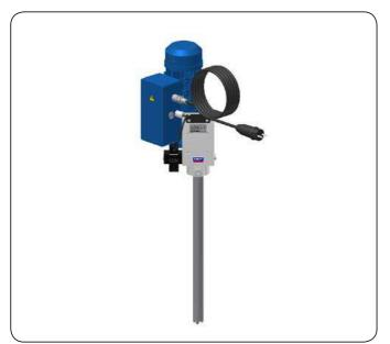
The EFFP electric grease feeding pump is a piston pump for grease drum sizes from 16 to 25 kg. The delivery stroke is generated at the lower end of the intake tube by a delivery piston that is controlled by an electrically driven eccentric shaft. The pump is activated using an ON/OFF switch attached to the terminal box.
